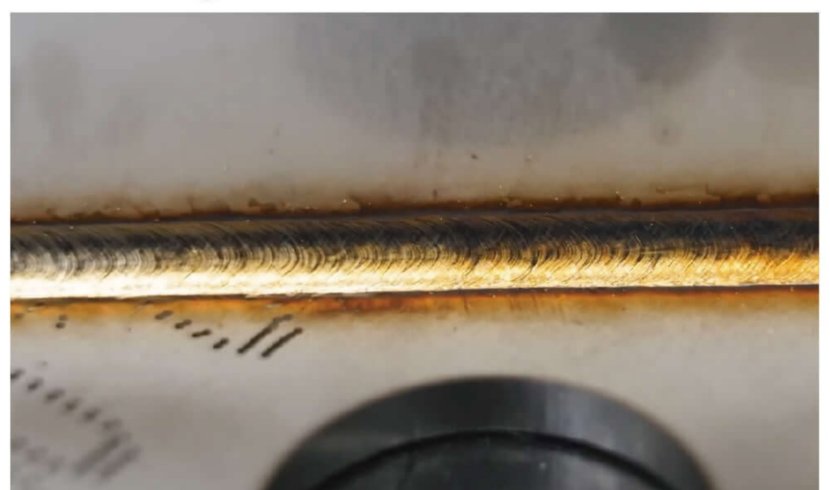
Welding with Filler
